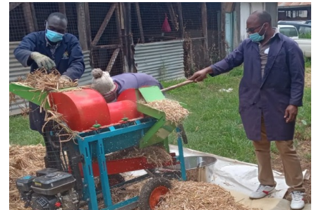
Fig 2: Testing of motorized legume thresher
