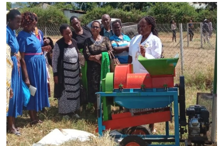
Fig 2: Testing of motorized legume thresher
